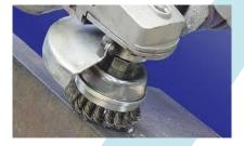
9) Power Tool Cleaning To Bare Metal (SSPC-SP11) - This type of surface preparation utilize the same equipment as Power Tool Cleaning to remove all visible coatings and contaminants to bare metal substrate.
