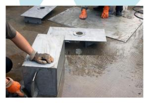
7) Hand Tool Cleaning (SSPC-SP2), (SSI-St2) - This is a mechanical method of surface preparation involving wire brushing, scraping, chipping and sanding.
